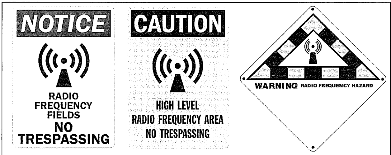
Figure 2. Typical Warning Signs for Radiofrequency Radiation
